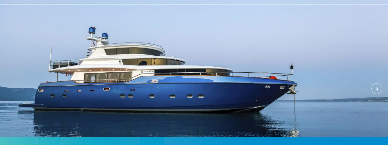
Loa 26.54m (87' 07") Beam 7.16m (23' 49") Draft 1.98m (6' 5") Built 2006 Refit 2013 Shipyard Johnson Yachts LTD Guests 10 Cabins 5 Crew 4 Speed 16 Knots
