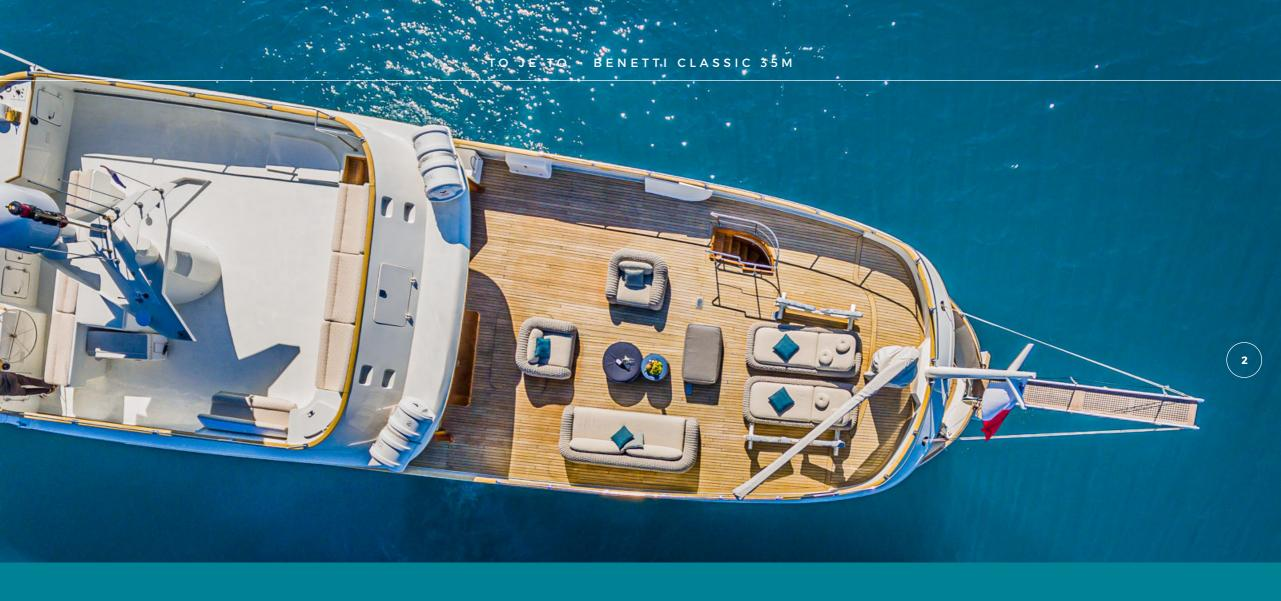
Loa **35,05 m (115' 0")** Beam **7.62 m (25' 0")** Draft **2.9 m (9' 6")** Built **1980** Refit **2022** Crew **5**Guests **8** Cabins **4 Builder** Benetti **Naval Architect** Stefano Righini **Hull Construction** Steel **Hull Configuration** Semi displacement
