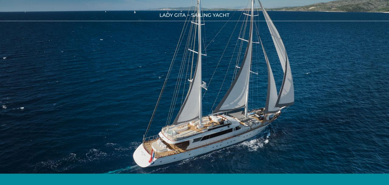
Loa 49.26 m (161' 7") Beam 8.66 m (28' 5") Draft 3.6 m (11' 10") Built 2019 Refit 2024 Guests 12 Crew 9 Builder Odisej d.o.o. Naval Architect Nauta Ltd, Split, Croatia Hull Material Steel Hull Configuration Displacement Yacht type Motor-sailer
