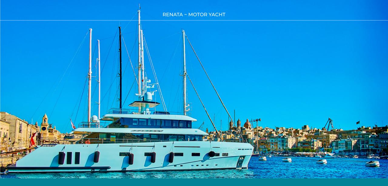
Loa **40.80 m (133' 10")** Beam **9.00 m (29' 6")** Draft **2.6 m (8' 6")** Built **2025** Guests **12** Crew **9**Naval Architect **Studio Sculli** Hull Material **Steel** Hull Configuration **Displacement** Superstructure **Flybridge**
